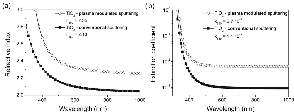
Fig. 7. Refractive index (a) and extinction coefficient (b) spectra of TiO<sub>2</sub> deposited by conventional and modulated plasma magnetron sputtering.
