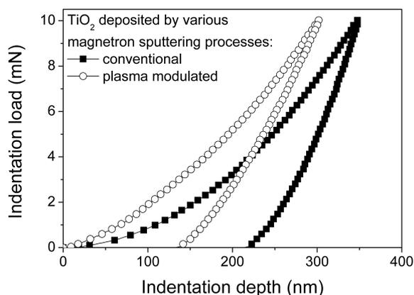
Fig. 3. Indentation load-depth curves of TiO<sub>2</sub> thin films deposited by various magnetron sputtering processes.
