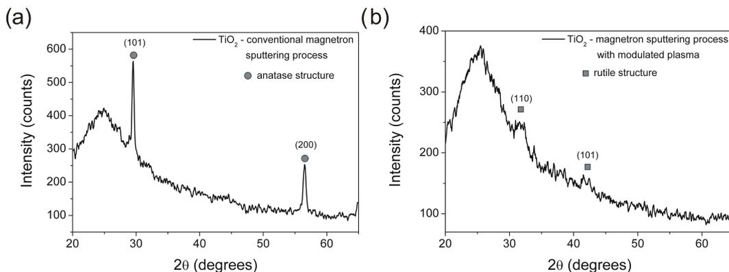
Fig. 2. XRD measurements results of TiO<sub>2</sub> deposited by (a) conventional and (b) modulated plasma magnetron sputtering processes [42, 43].
