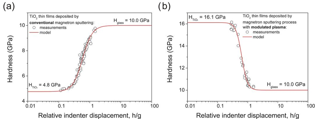
Fig. 4. Results of hardness measurements of  $\text{TiO}_2$  deposited by (a) conventional and (b) modulated plasma magnetron sputtering processes. The points show nanoindentation measurement results, and solid curves best fits to equations 1 and 2.
