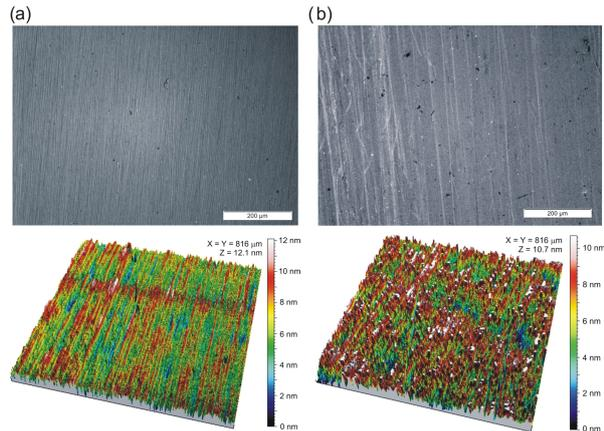
Fig. 5. Optical microscope and profilometer images of thin film surface after scratch tests of  $\text{TiO}_2$  thin films deposited by (a) conventional and (b) modulated plasma magnetron sputtering.
