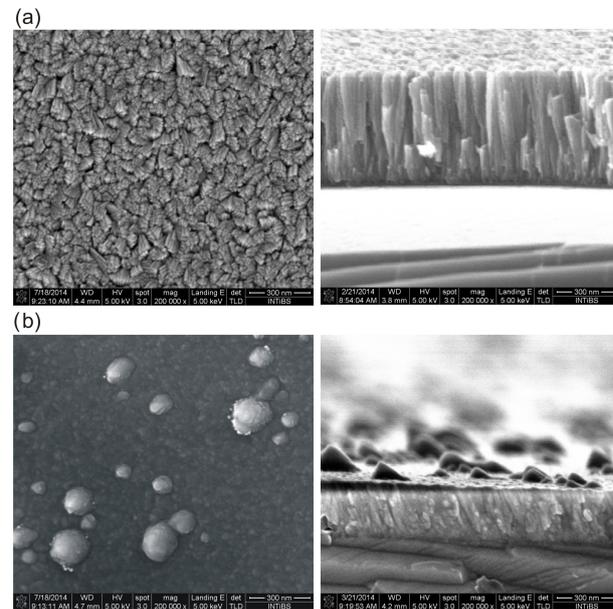
Fig. 1. SEM images of the surface (left side) and cross section (right side) of TiO<sub>2</sub> thin films deposited by (a) conventional and (b) modulated plasma magnetron sputtering processes.
