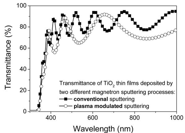
Fig. 6. Comparison of transmittance spectra of  $\text{TiO}_2$  deposited by different magnetron sputtering processes.
