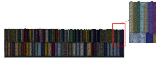
Fig. 9. Finite element discretization made on the Ti/TiN nanolayers.
