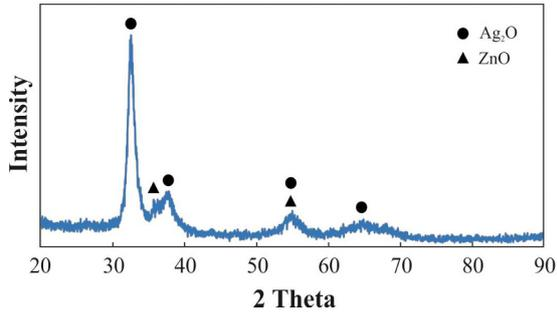
Fig. 2. XRD patterns of the milled powders.
