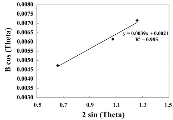
Fig. 4. Plot of  $\beta_S \cos \theta$  versus  $2 \sin \theta$  and the linear fit to the data.
