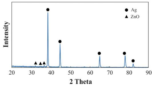
Fig. 3. XRD patterns of the heat treated powders.
