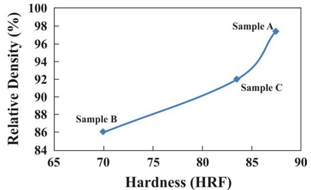
Fig. 6. Relative density versus hardness for the hot pressed compacts.
