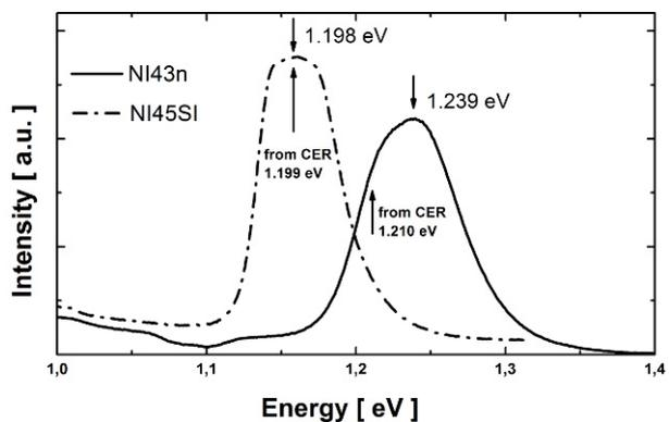
Fig. 2. PL spectra of the #NI43n and #NI45SI samples containing  $3 \times \text{InGaAsN}/\text{GaAs}$  QWs with marked first CER resonance energy.
