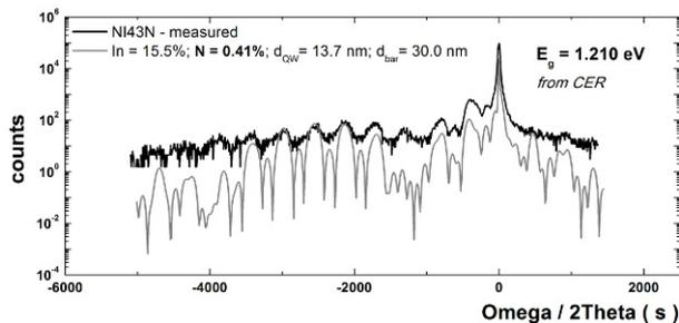
Fig. 6. (004)  $\omega/2\theta$  diffraction rocking curve of the #NI43n 3  $\times$  InGaAsN/GaAs MQW structure.
