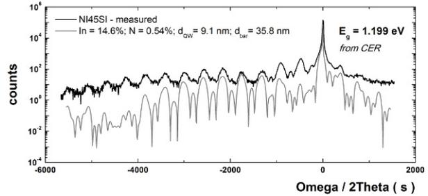
Fig. 7. (004)  $\omega/2\theta$  diffraction rocking curve of #NI45SI 3  $\times$  InGaAsN/GaAs MQW structure.
