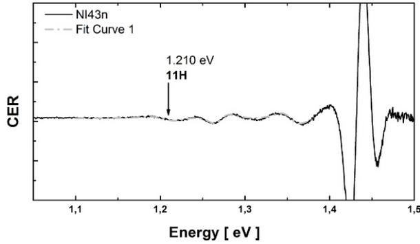
Fig. 3. CER spectrum of the #NI43n samples containing  $3 \times$  InGaAsN/GaAs QWs grown on the n-type (100) GaAs substrate with marked first QWs resonance.
