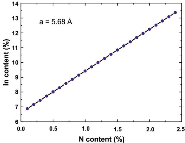
Fig. 1. Different combinations of indium and nitrogen contents for the InGaAsN lattice constant of 5.68 Å.
