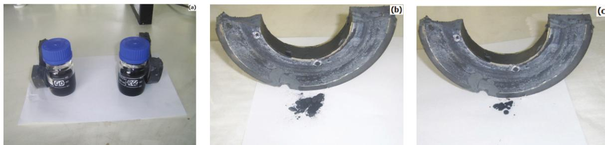
Fig. 7. Exposure to magnetic field from a semicircular magnet, (a) solution of graphene oxide and reduced graphene oxide (b) powdered graphene oxide and (c) powdered reduced graphene oxide.
