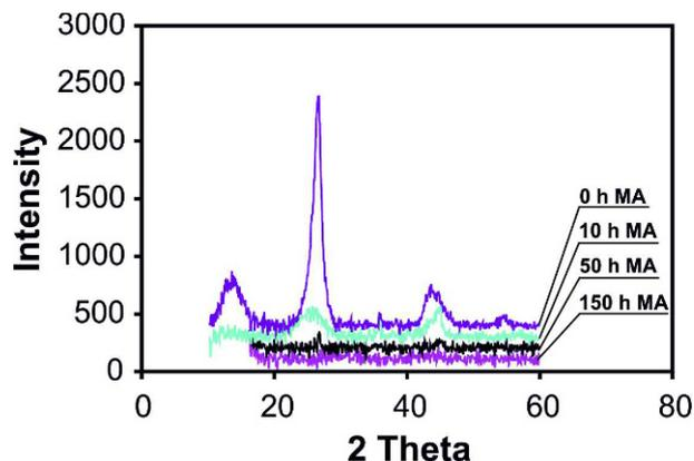
Fig. 1. The X-ray diffraction spectra of mechanically alloyed graphite powders at different milling times with 2 theta angle ranging from 10 to 60°.
