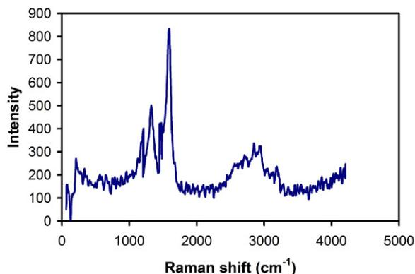
Fig. 5. Raman spectra of the MWCNTs obtained by mechanical activation.
