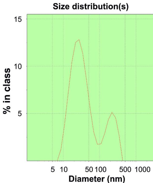
Fig. 2. The nanoparticle sizes of milled carbon measured by zeta-sizer.
