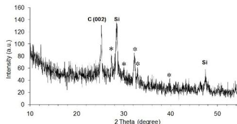
Fig. 6. X-ray diffraction measurements of carbon microstructures (discharge current  $i = 1.8$  mA, voltage  $U = 1$  kV, concentration 4 at.%  $C_6H_{12}$ ).
