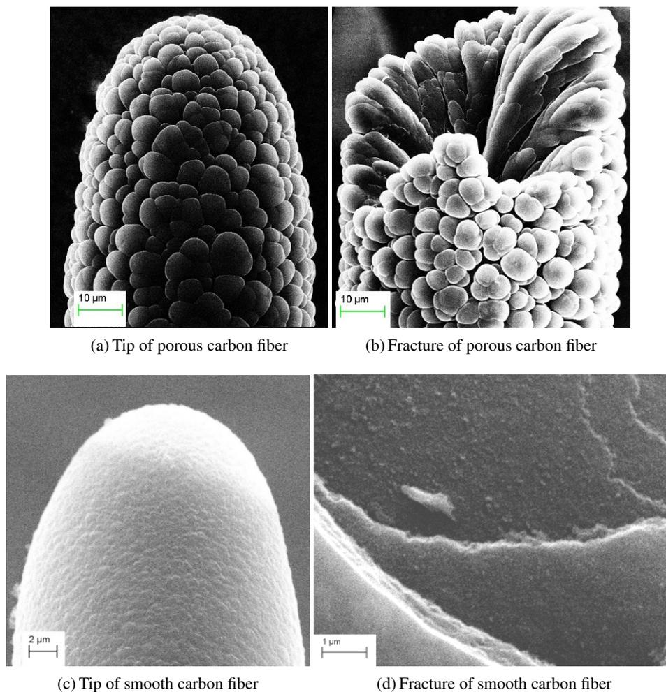
Fig. 3. SEM micrographs of carbon microfibers synthesised at the tip of the discharge electrode. Time of the synthesis of carbon structures: for (a) and (b) - 10 min,  $C_6H_{12}$  concentration - 1 at.%, and for (b) and (c) 30 s,  $C_6H_{12}$  concentration - 5 at.%; discharge current - 1.8 mA, voltage between the electrodes about 1 kV.
