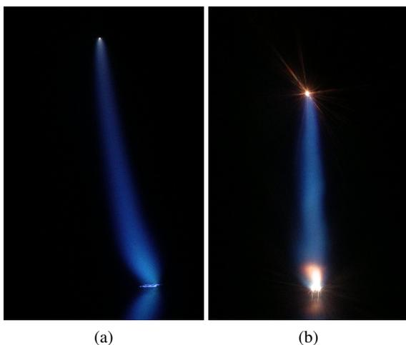
Fig. 2. Photographs of the discharge in Ar:C<sub>6</sub>H<sub>12</sub> (4 at.%) gas mixture for positive polarity; (a) discharge just after switching-on the voltage, (b) discharge during the synthesis of the carbon structures (1/100 s); discharge current: 1.8 mA, voltage drop between the electrodes: 2.25 kV.
