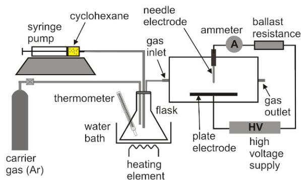
Fig. 1. Schematic of experimental set-up for the production of carbon microstructures.
