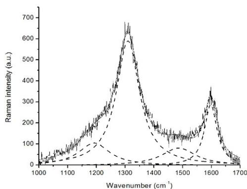
Fig. 5. Raman spectrum of carbon microstructures (solid line: experimental, dashed line: results of deconvolution) (discharge current  $i = 1.8$  mA, voltage  $U = 1$  kV, concentration 4 at.%  $C_6H_{12}$ ).
