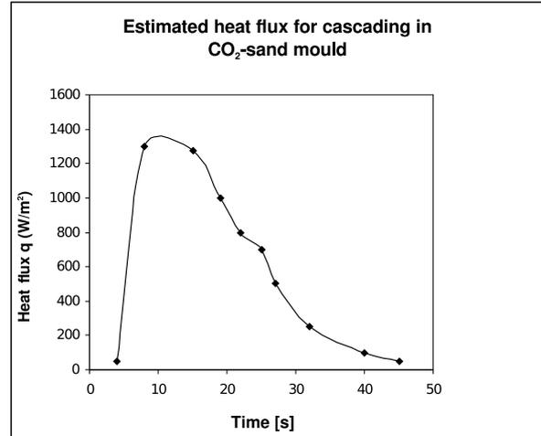
Fig. 9. Heat flux transients during solidification of Al-4.5 % Cu alloy in  $\text{CO}_2$ -sand moulds for 25 mm thickness (75 mm OD, 25 mm ID).
