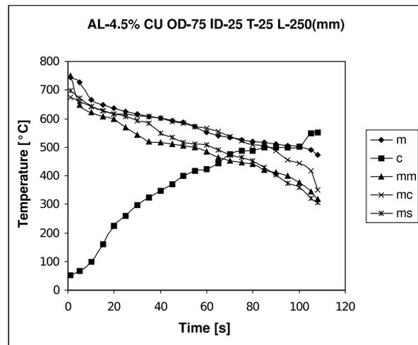
Fig. 3. Experimental cooling curves for 25 mm thickness (75 mm OD, 25 mm ID).
