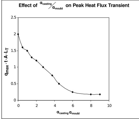
Fig. 7. Effect of  $\alpha_{\text{casting}}/\alpha_{\text{mould}}$  on peak heat transients for 25 mm thickness (75 mm OD, 25 mm ID).
