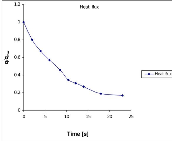
Fig. 8. Variation of normalized heat flux transient with time for 25 mm thickness (75 mm OD, 25 mm ID).
