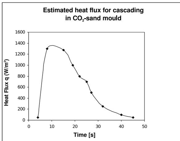
Fig. 5. Heat flux transients estimated by inverse analysis during solidification of Al-4.5 % Cu alloy in  $CO_2$ -sand mould for 25 mm thickness (75 mm OD, 25 mm ID).
