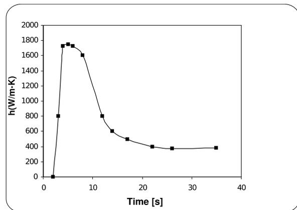
Fig. 6. Casting/Mould interfacial heat transfer coefficient for Al-4.5 % Cu alloy solidifying in  $CO_2$ -sand mould of 25 mm thickness (75 mm OD, 25 mm ID).
