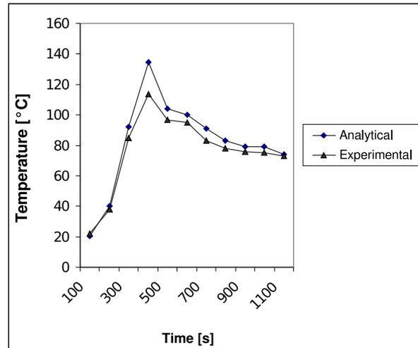
Fig. 2. Experimental and analytical temperatures inside CO<sub>2</sub>-sand mould 25 mm thickness (75 mm OD, 25 mm ID).
