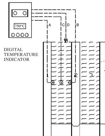
Fig. 1. Experimental set-up and thermocouples locations.
