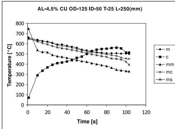
Fig. 4. Experimental cooling curves for 25 mm thickness (125 mm OD, 50 mm ID)
