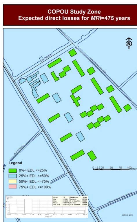
Fig. 8 - Expected direct structural losses of North area buildings for MRI=475 years earthquake
