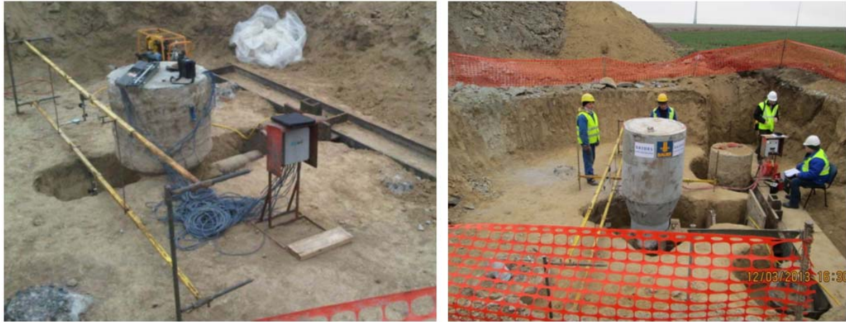
Fig. 5 – Static lateral load tests performance at TP1 and TP3 sites
