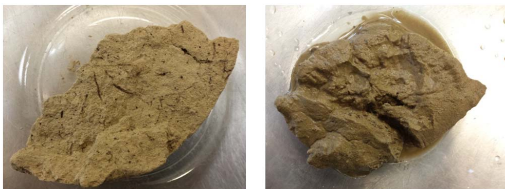
Fig. 1 – Sample of loess before and after the addition of water - collapse of structure
