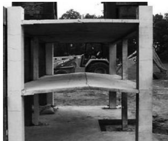
Fig. 4 - Residual deformation of the slab above the ground floor [7-8]
