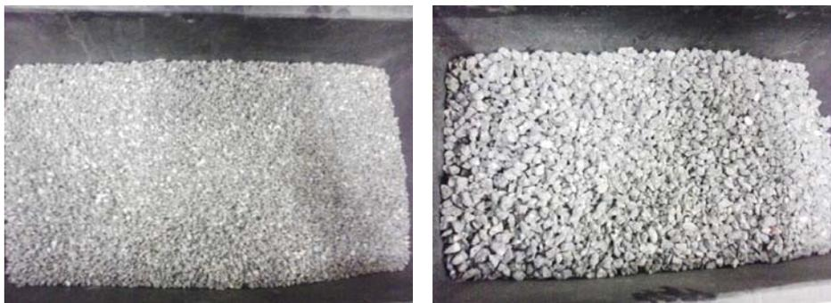
Fig. 1-2 The recycled aggregates, sorts 4-8 and 8-16
