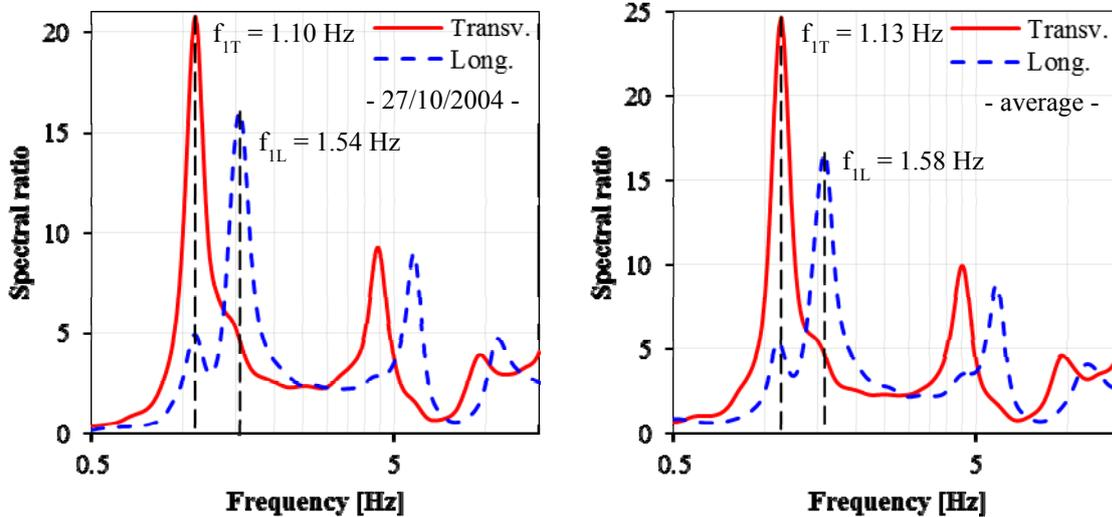
Fig. 6 – Spectral ratios for the 27/10/2004 ( $M_w = 6.0$ ) earthquake and average spectral ratios
