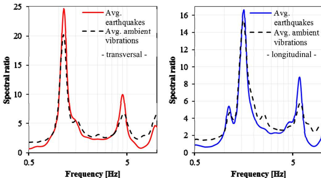
**Fig. 8** – Comparisons between average ambient vibrations spectral ratios and average seismic spectral ratios
