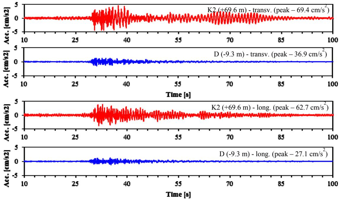
Fig. Error! No text of specified style in document. – Horizontal acceleration records at top and basement of BRD building
