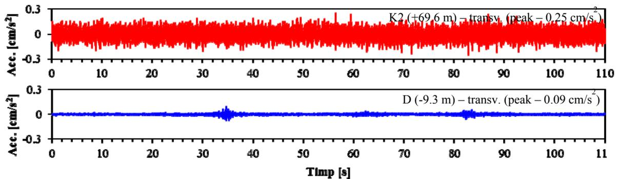
**Fig. 7** – Ambient vibrations recorded at the top and basement of the BRD building, transversal direction
