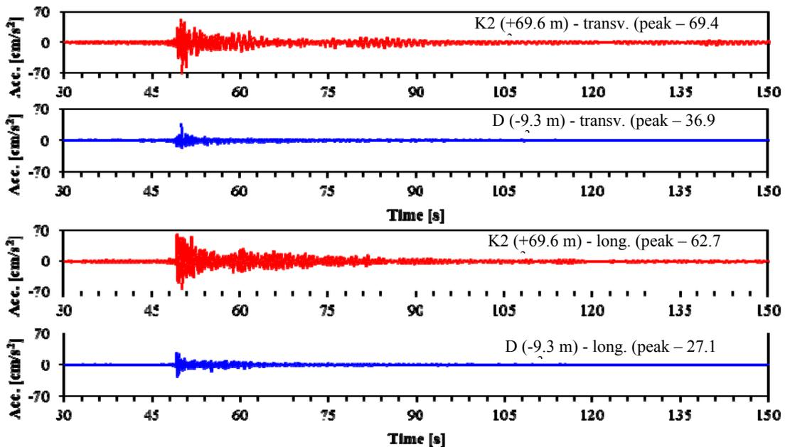
Fig. 3 – Horizontal acceleration records at top and basement of BRD building (27/10/2004 subcrustal Vrancea earthquake,  $M_W = 6.0$ )
