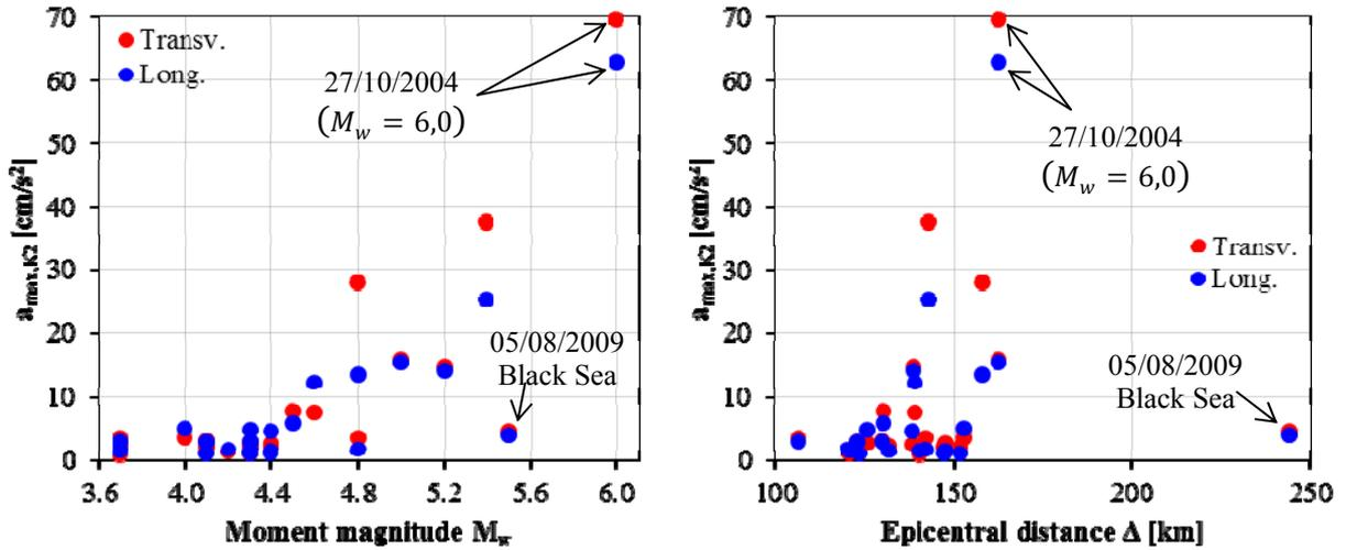
Fig. 2 – Variation of the peak accelerations recorded at the top of the BRD-SG building with earthquake magnitude and epicentral distance
