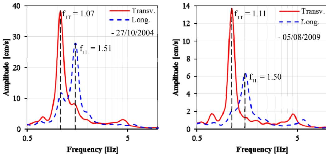
Fig. 5 – Fourier amplitude spectra of the top motions recorded during 27/10/2004 ( $M_W = 6.0$ ) and 05/08/2009 ( $M_W = 5.5$ ) earthquakes
