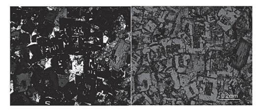
Fig. 7. Micropegnatitic aggregates in lamprophyres.
