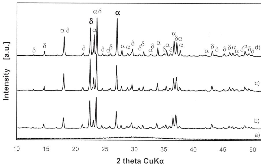
Fig. 1. XRD patterns of samples prepared according to method A, showing the influence of the calcination time at  $700^\circ\text{C}$ :
