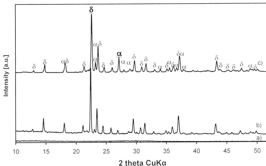
Fig. 5. XRD patterns of samples prepared according to method B, showing the influence of the calcination time at 700°C: a) amorphous  $\text{Na}_2\text{Si}_2\text{O}_5$  dried at 100°C obtained according to method B, b)  $\text{Na}_2\text{Si}_2\text{O}_5(700,1)\text{-B}$ , c)  $\text{Na}_2\text{Si}_2\text{O}_5(700,5.5)\text{-B}$  (reflections belonging to the  $\delta$  and  $\alpha$  phases are marked, those used for determination of relative contributions are underlined)
