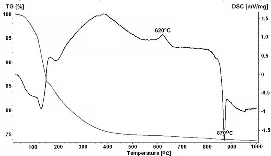
Fig. 2. TG/DSC analysis profiles of amorphous  $\text{Na}_2\text{Si}_2\text{O}_5$  obtained according to method A
