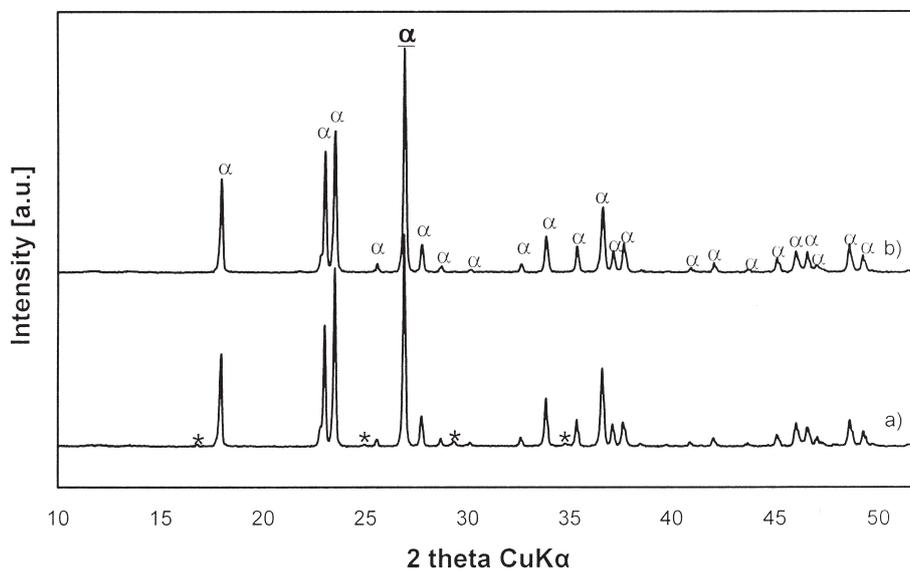
Fig. 3. XRD patterns of the materials prepared according to method A and calcined for 24 h at 825°C, showing the influence of the use of double volume of solvents:
