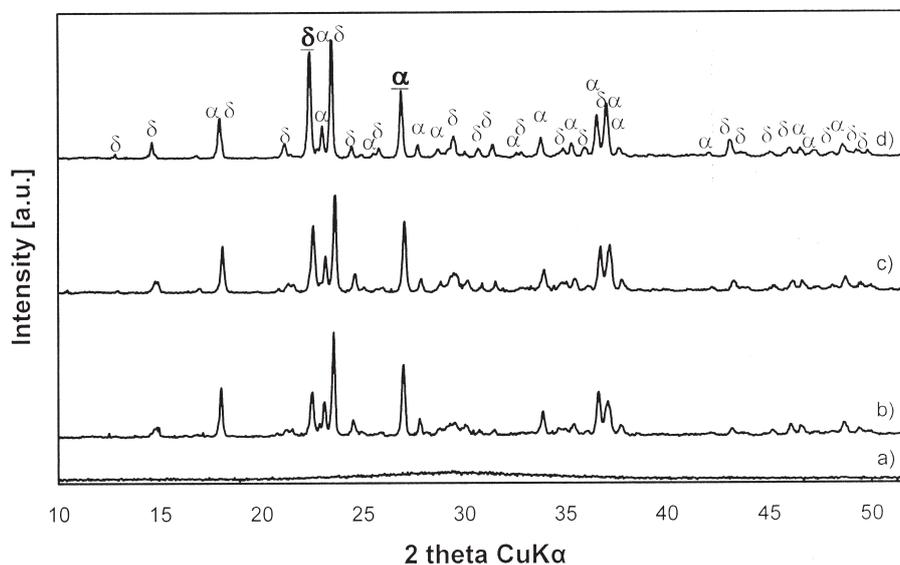
Fig. 4. XRD patterns of samples prepared according to method A and calcined for 1 h at different temperatures: a)  $\text{Na}_2\text{Si}_2\text{O}_5(450,1)\text{-A}$ , b)  $\text{Na}_2\text{Si}_2\text{O}_5(550,1)\text{-A}$ , c)  $\text{Na}_2\text{Si}_2\text{O}_5(620,1)\text{-A}$ , and d)  $\text{Na}_2\text{Si}_2\text{O}_5(700,1)\text{-A}$  (reflections belonging to the  $\delta$  and  $\alpha$  phases are marked respectively, those used for determination of relative contributions are underlined)
