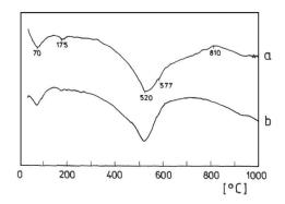
Fig. 2. DTA curves of the Triassic red clay of the Kozów deposit (sample 873) before (a) and after (b) removal of organic matter
