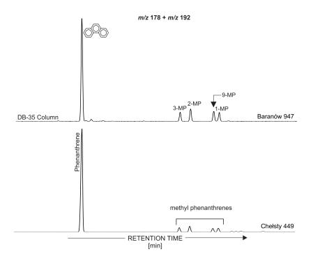
Fig. 5. Partial mass chromatograms showing distribution of phenanthrene and methyl phenanthrenes (m/z1 78 + 192) in clays from Chełsty and Baranów open pits (aromatic fraction)
