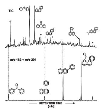
Fig. 3. Partial mass chromatogram showing distribution of benzophenone (m/z 182) and phenylnaphthalenes + cyclopenta(*def*)phenanthrenone (m/z 204) in green clay from the Chełsty open pit (polar fraction). DB-5MS column was used
