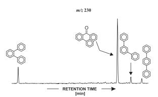
Fig. 4. Partial mass chromatogram showing distribution of terphenyls and benzanthrone (m/z 230) in green clay from the Chełsty open pit (polar fraction). DB-5MS column was used
