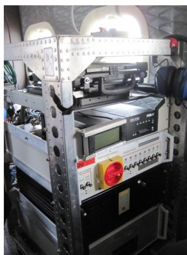
Figure 1. APEX instrument and computer rack installed in the aircraft (photo credits: Bart Bomans and Johan Mijndonckx, VITO)
