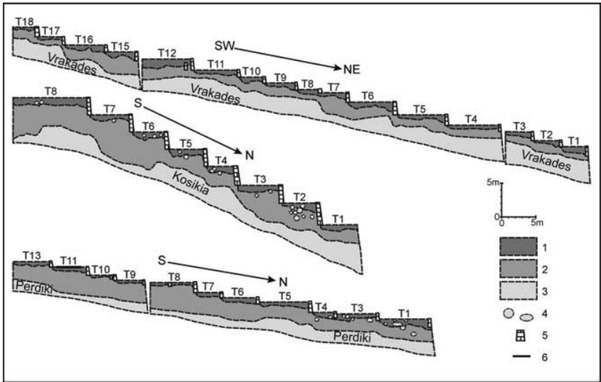
Fig. 6. The interpretation of selected georadar profiles. Their course was marked on Fig. 5
