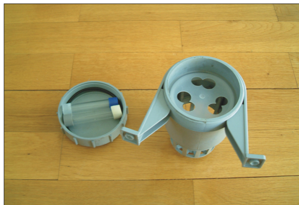
Fig. 2: Diffusive samplers and shelter (Photo: M. Ogrin)
