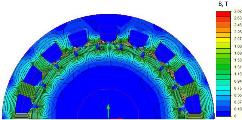
*Fig. 2. Magnetic field in the PMSG cross-section.*
