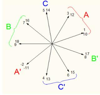
Fig. 3. Vector diagram of PMSG electromotive forces.
