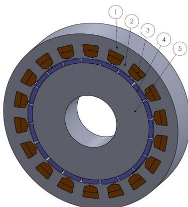
Fig. 1. Cross-section of a PM generator with  $Z_1/2p = 18/20$ :
