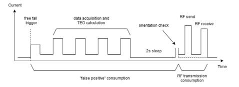
Fig.3. Device active mode current consumption explanation.
