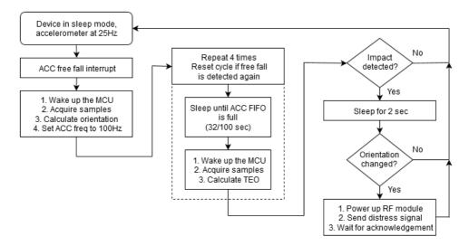
Fig. 2. Fall detection algorithm.
