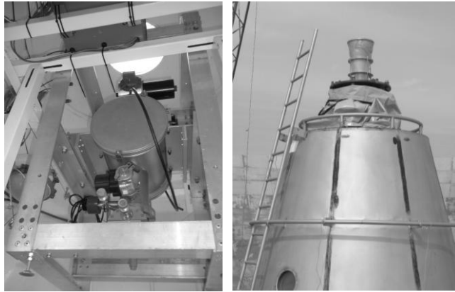
Fig. 3. The receiver system for the 5 GHz frequency band: cryogenic receiver mounted in the secondary focal room (left) and connected with a waveguide to the feedhorn in the secondary focus of radiotelescope RT-32 (the right).
