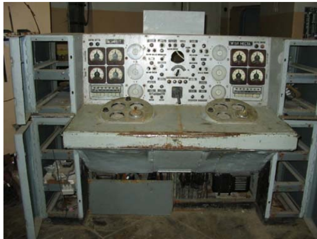
Fig. 8. The control panel (originally used to operate the antenna manually).
