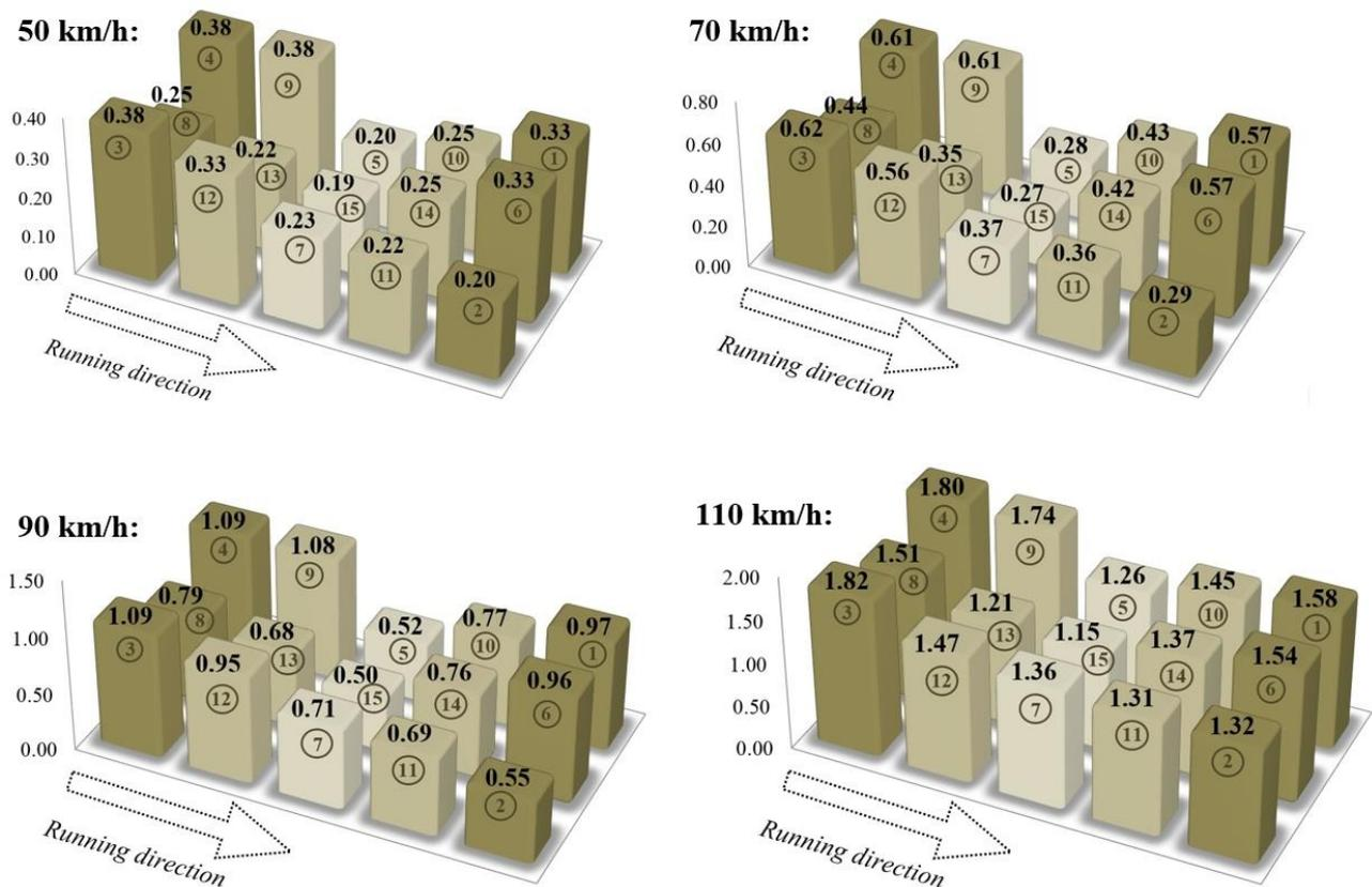
**Fig. 4** Location of measured points for the assessment of a passenger ride comfort. Source: authors
