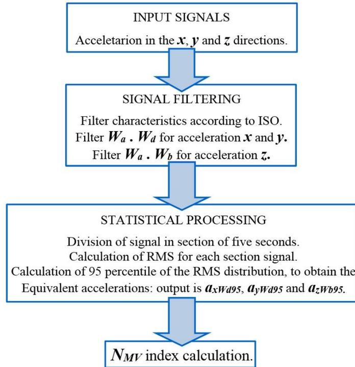
**Fig. 2** Process of the  $N_{MV}$  comfort index calculation. Source: [1,8]
