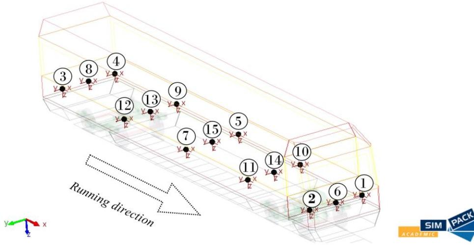
**Fig. 3** Location of measured points for the assessment of a passenger ride comfort. Source: authors
