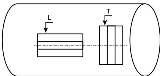
Fig. 1. The scheme of obtaining specimens on the tensile test
