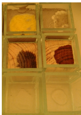
Figure 3: Acid spills on concrete, wood and glass
