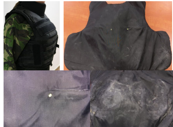
Figure 4. Results of ballistic tests a. Ergonomic female bulletproof vest (before tests), b. shooting views on ballistic package, c. bust impact (detail), d. back of ballistic package (detail).
