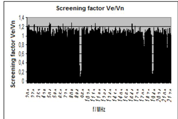
Fig. 2 The screening factor representation for a radio-absorbing material screen
