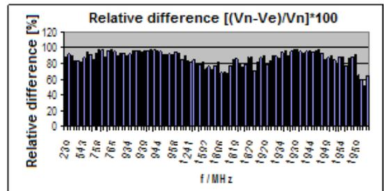
Fig.8 The variation of the relative damping related to frequency, on the poop deck
