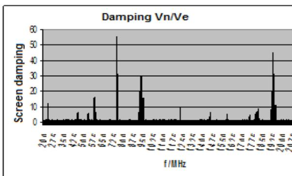
Fig.1 The damping representation for a radio-absorbing material screen
