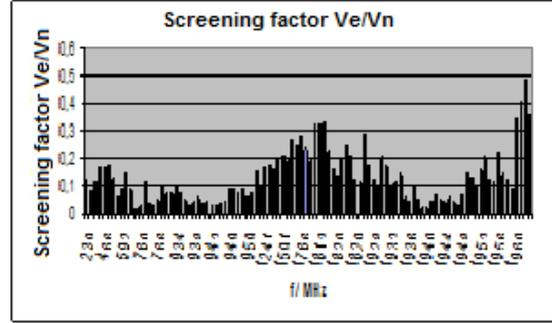
Fig.7 The representation of the screening factor for a screen made of radio-absorbing materials for the first 100 values of the intensity of the electric field
