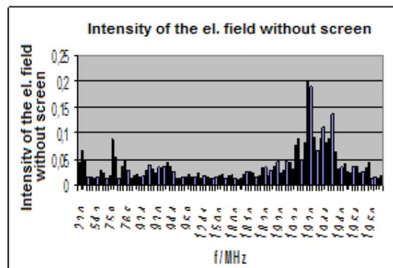
Fig.3 The representation of the first 100 values of the electric field with the station emitting from the poop deck on the frequency of 240 MHz, without screen
