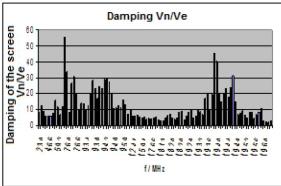
Fig.5 The representation of the damping of the screen made of radio-absorbing materials for the first 100 values of the intensity of the electric field
