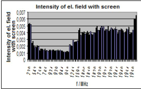
Fig.4 The representation of the first 100 values of the electric field with the station emitting from the poop deck on the frequency of 240 MHz, with screen
