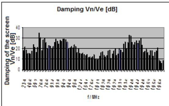
Fig.6 The representation of the damping of the screen made of radio-absorbing materials, in dB, for the first 100 values of the intensity of the electric field
