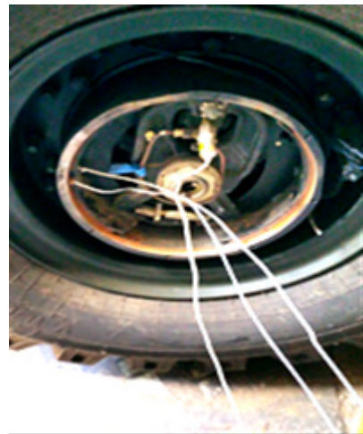
Figure 4: Installed sensors for taking the temperature of the brakes
