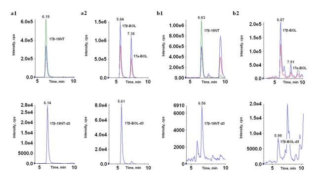
**Fig. 2.** LC-MS/MS extracted ion chromatograms (XIC) of 17β-19-nortestosterone and 17α/β-boldenone: a1), a2) in urine sample spiked at 10 µg L<sup>-1</sup>, b1), b2) in real urine sample from a pig confirmed at 69.1 µg L<sup>-1</sup> of 17β-19-nortestosterone, 10.8 µg L<sup>-1</sup> of 17β-boldenone, and 3.9 µg L<sup>-1</sup> of 17α-boldenone
