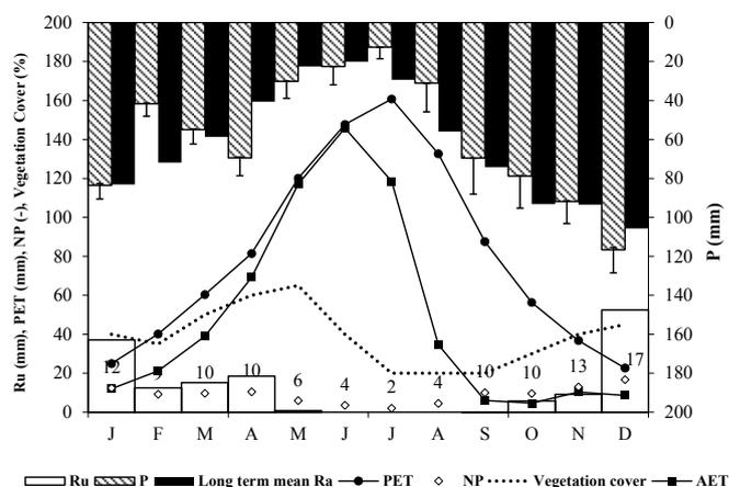
**Fig. 2.** Monthly mean values of precipitation depths ( $P$  and its standard deviation), number of rainy days ( $NRA$ ), potential evapotranspiration ( $PET$ ), actual evapotranspiration ( $AET$ ), runoff depths ( $Ru$ ) and Vegetation Cover observed at the Cannata watershed (1996–2006) and long term monthly mean  $P$  measured at the Randazzo pluviometric station.
