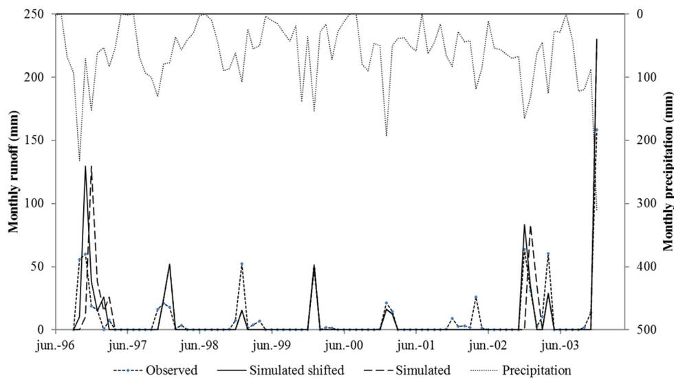
**Fig. 3.** Monthly precipitation *P* and runoff *Ru* observed and simulated with the T-M model.
