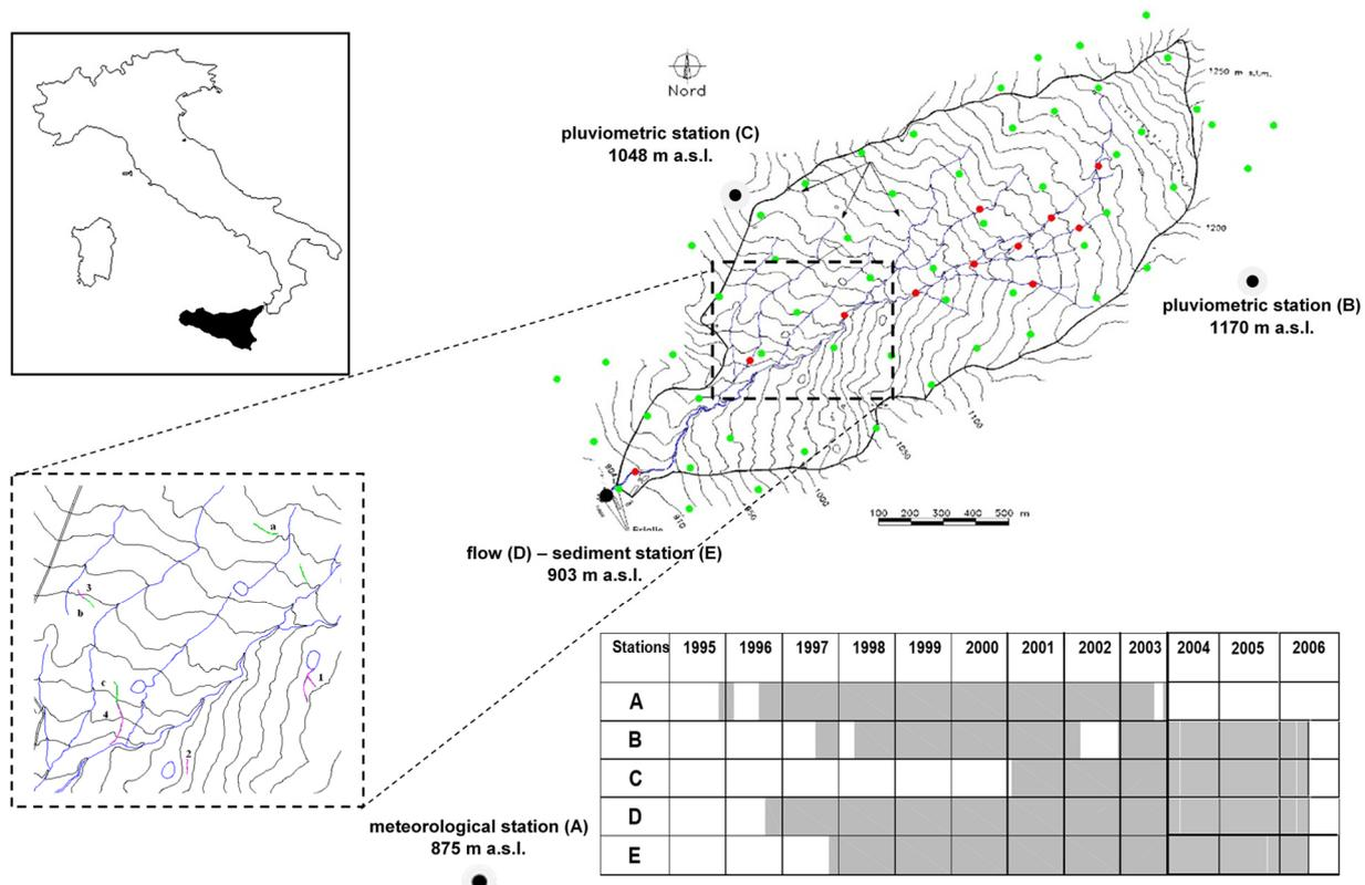
**Fig. 1.** Layout of sub-watersheds and hydrological network in the Cannata watershed, Sicily. Small dots indicate the location of soil samples. The figure enlargement on the left shows gully formations and small ponds for animal watering. The table shows the recording periods for the diverse stations.
