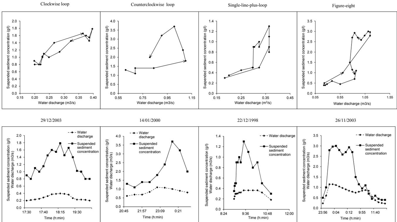
Fig. 5. Examples of suspended sediment concentration - water discharges relationships observed in the Cannata watershed.
