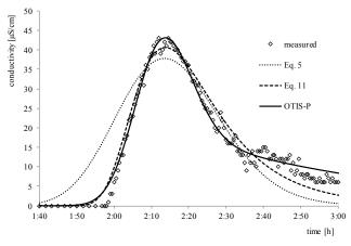
**Fig. 3.** Comparison of measured and simulated conductivity distribution in the test A - Malá Nitra stream, experiment Nr. 5-V (1340 m).
