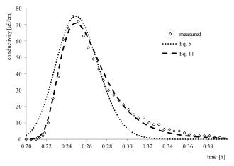
**Fig. 6.** Comparison of measured and simulated conductivity distribution in the selected profiles on the test B - Šúrsky stream, exp. Nr. 11-II (406 m).
