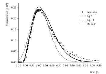
**Fig. 7.** Comparison of approximation results – test C, the Malina stream (approximation using Eq. (5) and Eq. (11) and the OTIS software).
