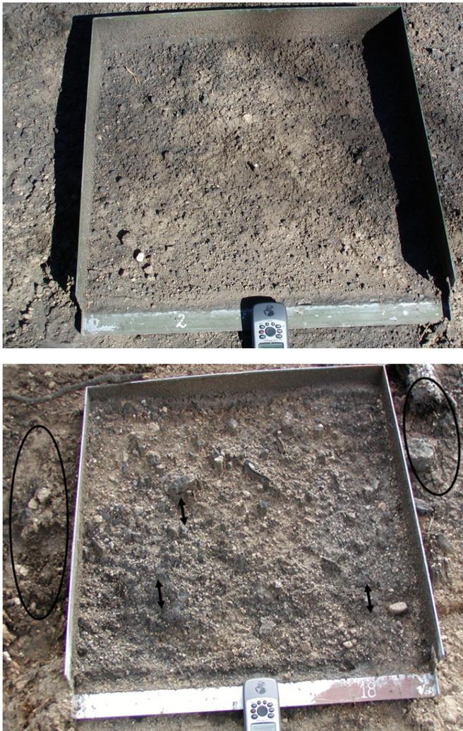
**Fig. 4.** Example plots from a) the burned 20% site, and b) the burned 60% site. The metal plot frames delineate the 0.5 m<sup>2</sup> plot area from which the runoff and sediment samples were taken. Black ovals on b) show the rocks and stumps on site which can indicate macropores and increased ponding, while arrows highlight the rougher soil surface texture which slows surface flow and may increase infiltration.
