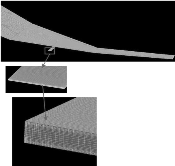
Fig. 3a. Fragment of the structural mesh with the boundary layer.
