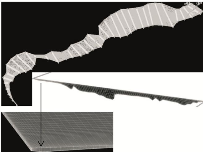
Fig. 3b. Example of the computational domain with the structural mesh for the whole domain and one cross-section; under magnification, hexahedral elements are included in the boundary layer.
