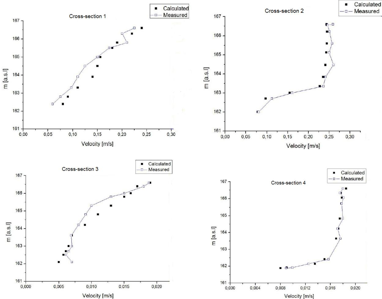
**Fig. 5.** Velocity profiles from time-averaged fixed boat ADCP measurement and CFD calculations.
