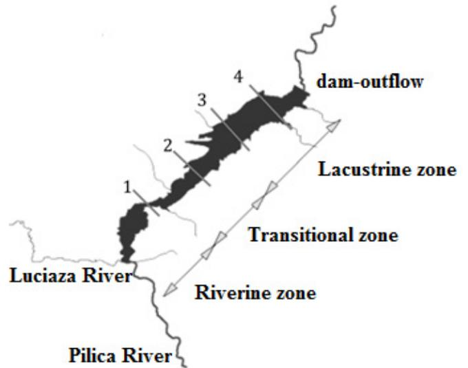
**Fig. 4.** Division of the Sulejow reservoir into riverine, transitional and lacustrine zones, with the locations used for model verification marked.
