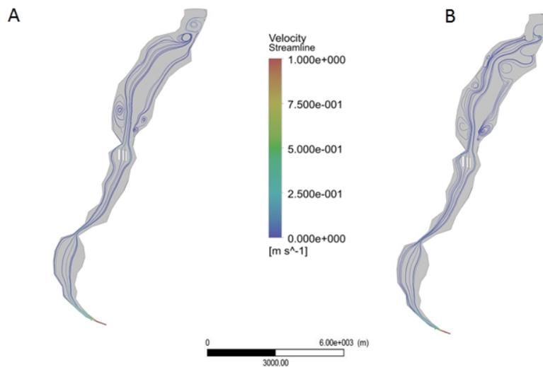
Fig. 7. Comparison of velocity field (m/s) in the Sulejow reservoir in October 2007 under wind and under no wind.
