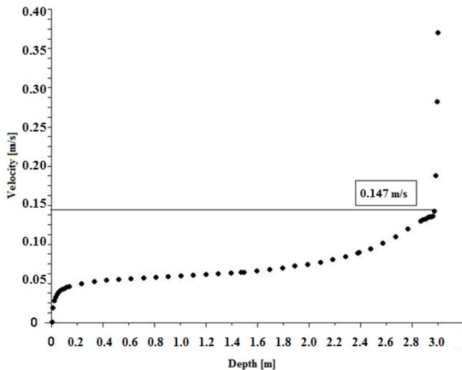
Fig. 1. The velocity profile of water at the outlet of the computational domain.
