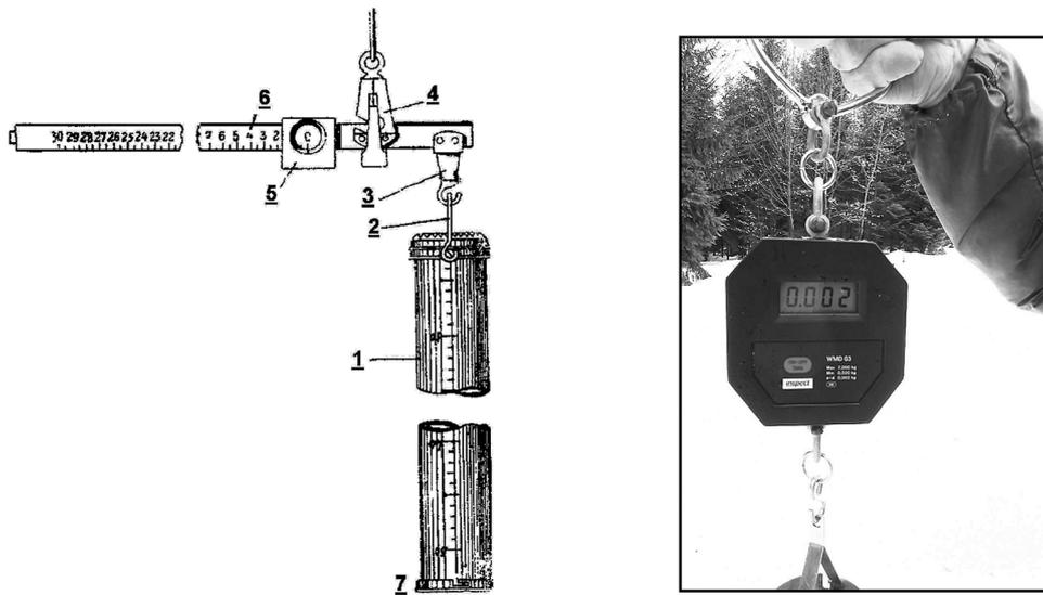
Fig. 3. On the left side: Snow gauge VS-43 (1 – sampling cylinder, 2 – grip, 3 – hook, 4 – hanging balance, 5 – balancing , 6 – arm of the unequal-armed balance, 7 – classic security lid); On the right side: Up-dated snow gauge with a digital balance.
