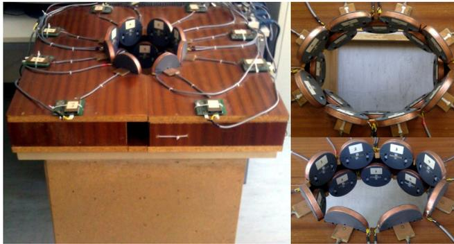
Fig. 3: The mechanical body and elliptical coil system of the used MITS tomograph. The two-plane transceiver array is fitted in a custom-built, robust wooden table which has some kind of opening mechanism that allows positioning a test person or a large test phantom into the coil system.
