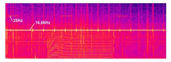
Fig. 7. A single "Cow" signal recorded during 20 minutes at the north of the mountains "Eifel", frequency vs time; colour — as amplitude
