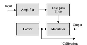
Fig. 3. Recording equipment via the sound card of the PC
