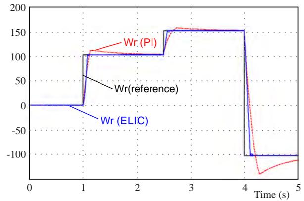
Fig. 7. Simulated speed responses of the drive due to step change of the reference speed ELIC and PI
