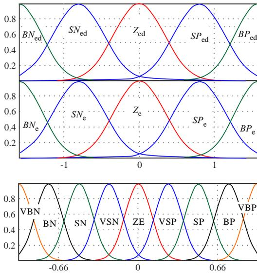
Fig. 5. Fuzzy critic membership functions: (a) – input membership functions and (b) – output membership functions
