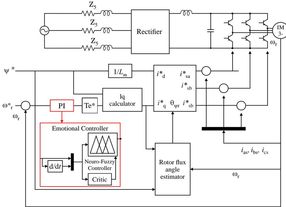
Fig. 1. The proposed emotional controller based IM drive
