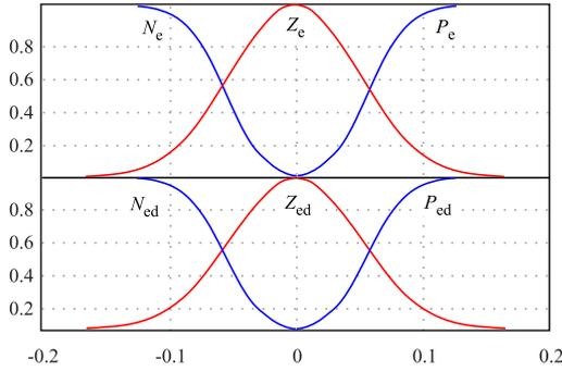
Fig. 4. The membership functions of the corresponding linguistic variables of the neuro-fuzzy Controller
