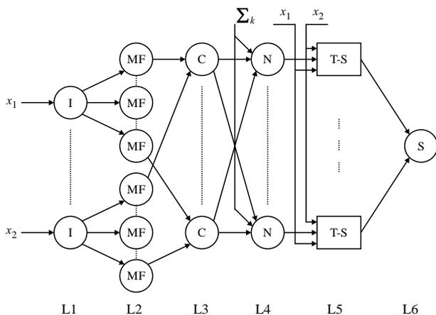
**Fig. 3.** Neuro-fuzzy structure equivalent with a MISO TSK fuzzy inference system with layers: L1 – input fuzzyfier, L2 – input linguistic, L3 – conjunction, L4 – normalizer, L5 – TSK rules and L6 – summation
