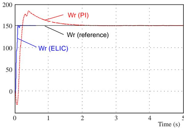
Fig. 6. Simulated starting responses of the drive with ELIC and PI
