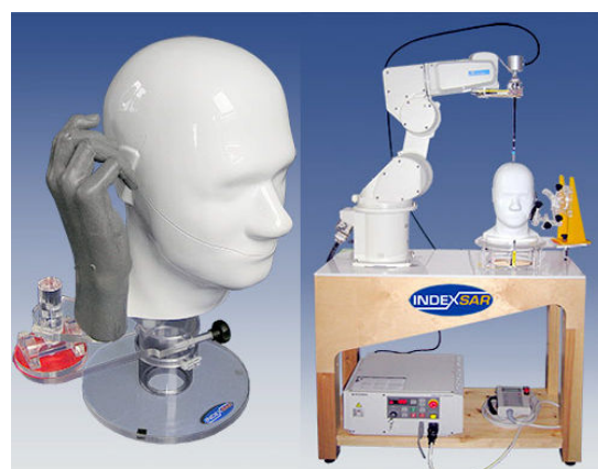
Fig. 1. Phantom model for SAR testing and determining radiation levels [10, 12]
