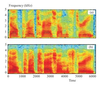
**Fig. 6.** Sectrogram of signal: (a) – before shifting the pitch, (b) – after the modification
