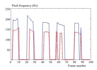
Fig. 9. Source pitch period per frame (solid line), and the new pitch period (dotted line)
