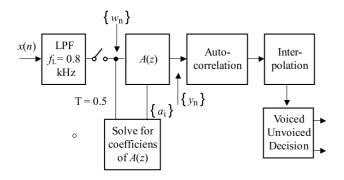
${\bf Fig.~3.}$  Block diagram of a simplified SIFT block diagram
