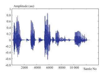
${f Fig.~5.}$  Speech signal waveform after channing the pitch
