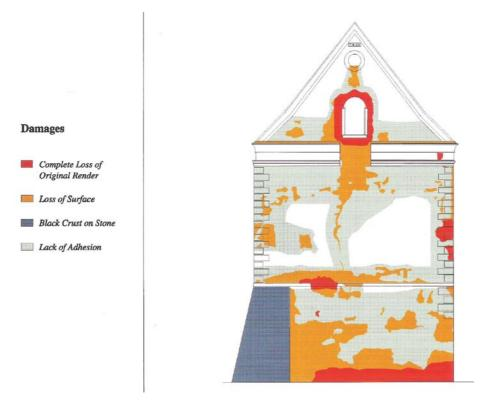
Figure 8. Display of a damage map (Kartause Mauerbach) [4]
