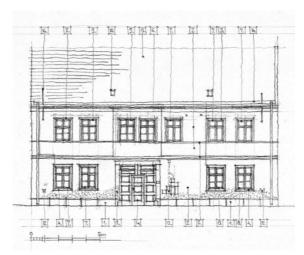
Figure 5. Condition recording façade drawing indicating defects (Sopron, Móricz Zsigmond Street)
