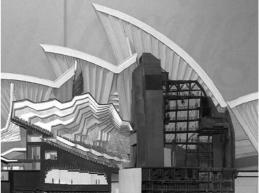
Figure 11. Utzon's proposal for the load bearing acoustic ceiling by undulating ply-wood beams using cylinder geometry
