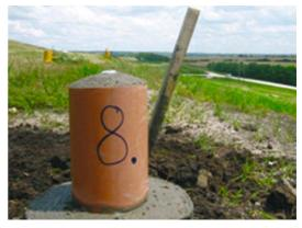
Figure 5. Settlement measuring point.
