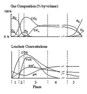
Figure 6. The anaerobic decomposition of organic matter ([9])
