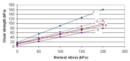
Figure 7. Shear strength results for degradation phase 1 to 5 (after [7])
