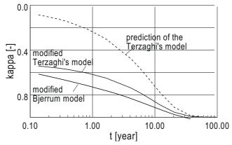
Figure 17. The different time dependency of the self-weight settlement by the various models.
