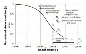
Figure 16. The approximate value of the waste shear modulus  $G_1$  and  $G_2$  determined from the waste oedometric modulus (computed from the primary consolidation settlement  $(E_1)$  and from the sum of the primary consolidation settlement and the creep settlements  $(E_2)$ ) with respect to the small strain shear modulus  $G_0$  measured by seismic test.  $(G_2, G_3$  are too small to illustrate on the figure)
