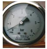
(f) the lateral stress measuring gauges
