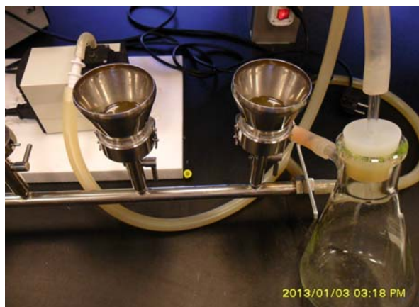
Figure 9: Filtering the measured mixture through 45 \mu\text{m} paper
