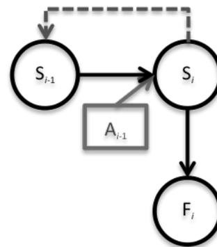
Figure 73: Generic single-slice trellis with an optional action.
