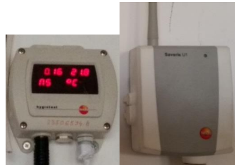
Figure 4. The central unit and the sensors of the system for recording measured data
