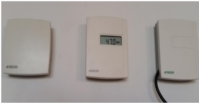
Figure 3. Interior drive sensors of the natural ventilation system
