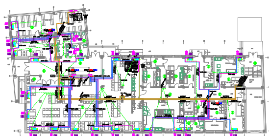
Figure 2. Ground floor heating / cooling system
