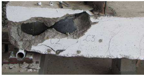
Figure 1. Failure at shear force – DG3 slab
