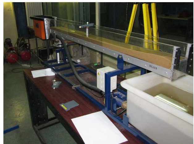
Figure 3. Scheme of sediment transport demo channel (Craciun, 2014)
